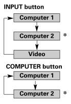
Computer 2 is not displayed when the RGB IN-2/ COMPO-NENT IN/ RGB OUT terminal is used as Monitor out.
