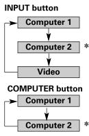
Computer 2 is not displayed when the RGB IN-2/ COM-PONETN IN/ RGB OUT terminal is used as Monitor out.
